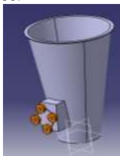
Fig. 4.3 3D cad model of bucket with rollers
